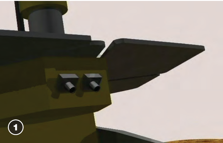
The autonavigation system takes left and right pictures of the nearby terrain using the Mars Exploration Rover body-mounted stereo hazard-avoidance cameras or mast-mounted stereo navigation cameras.
