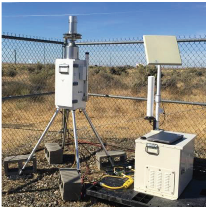
An Environmental Continuous Air Monitor (ECAM) deployed in the field. For the Mars 2020 launch, 30 of these sophisticated environmental monitoring systems will be deployed in the area surrounding the launch site prior to launch. Credits: Department of Energy
