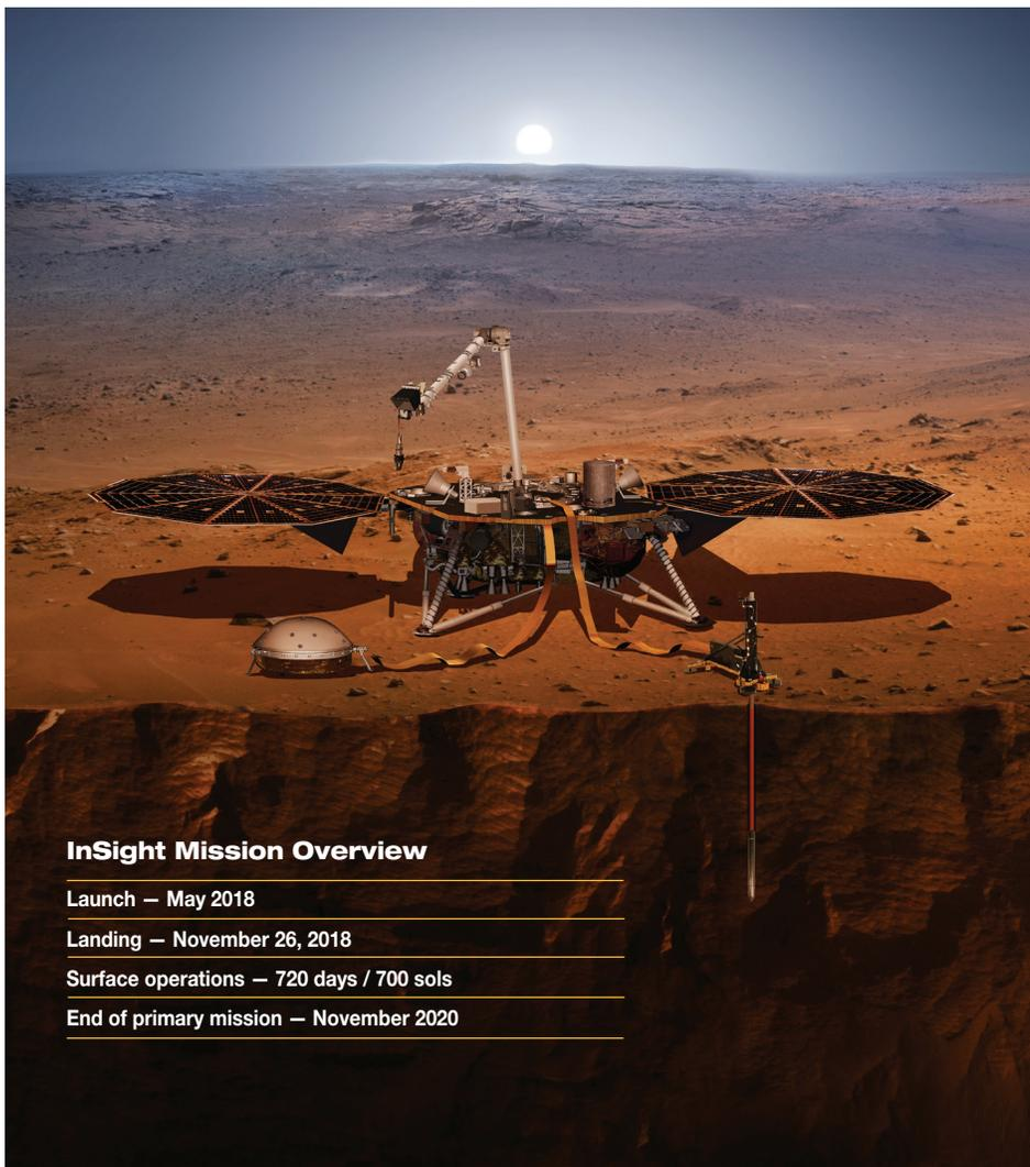
*InSight is based on the proven Phoenix Mars spacecraft and lander design with state-of-the-art avionics from the Mars Reconnaissance Orbiter and Gravity Recovery and Interior Laboratory missions.*
