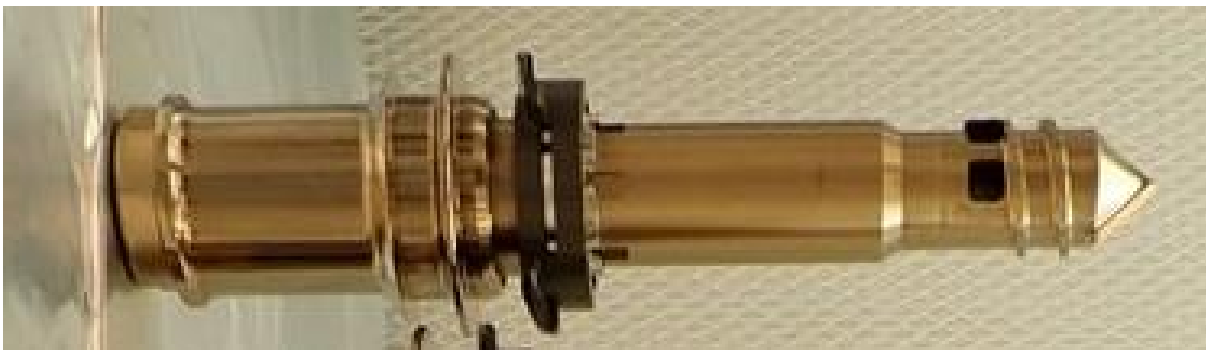
Figure 5 | Regolith sampling bit. The bit contains two windows that are each 8 mm tall x 7.4 mm wide.
