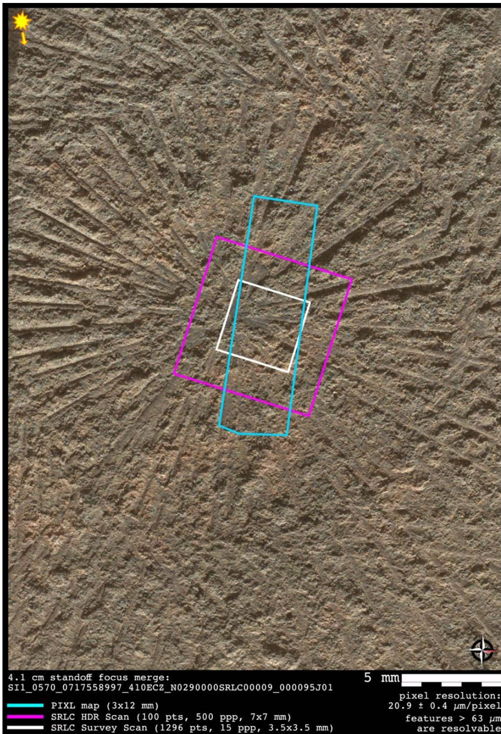
Figure 8 | WATSON post-abrasion focus merge from 4.1 cm standoff of the interior of the Novarupta abrasion with the footprints of the Sol 570 SHERLOC spectroscopy (pink, white) and PIXL map (cyan) analyses overlain. Sunlight illumination is from the upper left.
