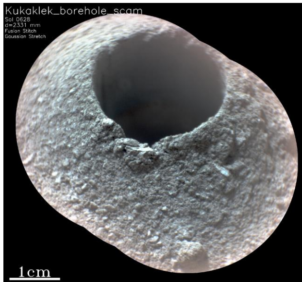
Figure 11 | SCAM RMI borehole image after Kukaklek core extraction (Sol 628).
