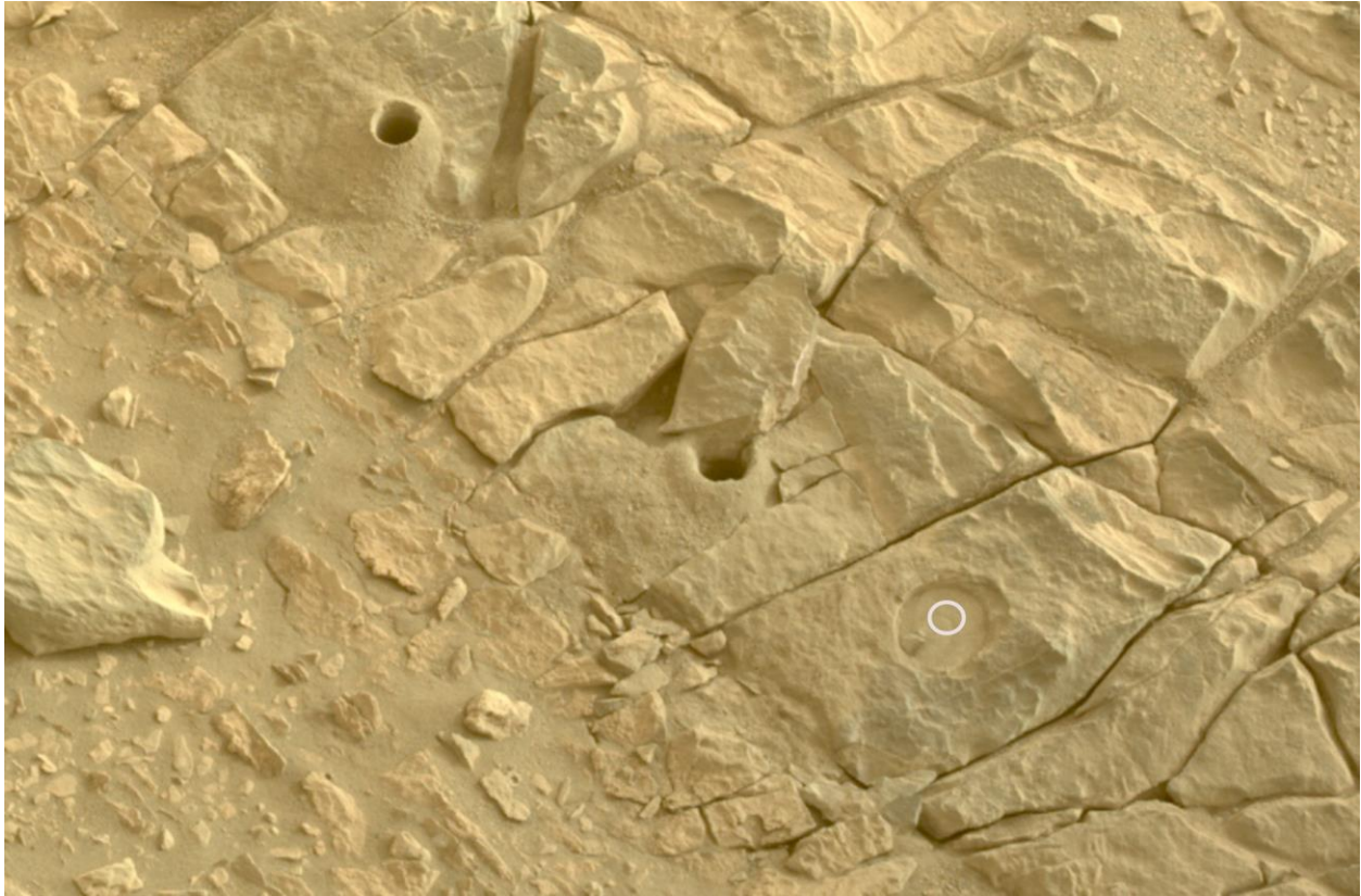
Figure 1 | Navcam left sol 579 mosaic showing Amalik with abrasion patch Novarupta and drill holes of Shuyak and Mageik . During simulated coring the drill was positioned directly above the white circle.
