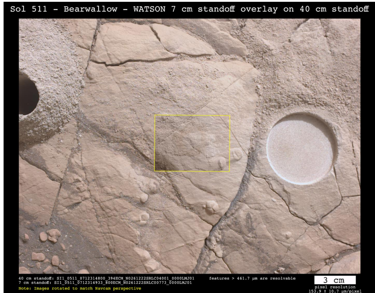
Figure 7 | Sol 511 WATSON 40 cm standoff image of Wildcat Ridge , showing the Berry Hollow abrasion patch (right) and the Hazeltop core tailings (left). The center inset is a WATSON 7 cm image inset of the Bearwallow target (pre-core).
