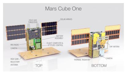
Illustration of the twin MarCO spacecraft with some key components labeled. The top cover is left out to show some internal components. Antennas and solar arrays are shown deployed. Image credit: NASA/JPL-Caltech
