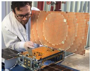
Engineer, Joel Steinkraus, uses sunlight to test the solar arrays on one of the MarCO spacecraft at NASA's Jet Propulsion Laboratory. Image credit: NASA/JPL-Caltech
