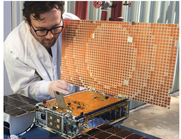
Engineer, Joel Steinkraus, uses sunlight to test the solar arrays on one of the MarCO spacecraft at NASA's Jet Propulsion Laboratory.
