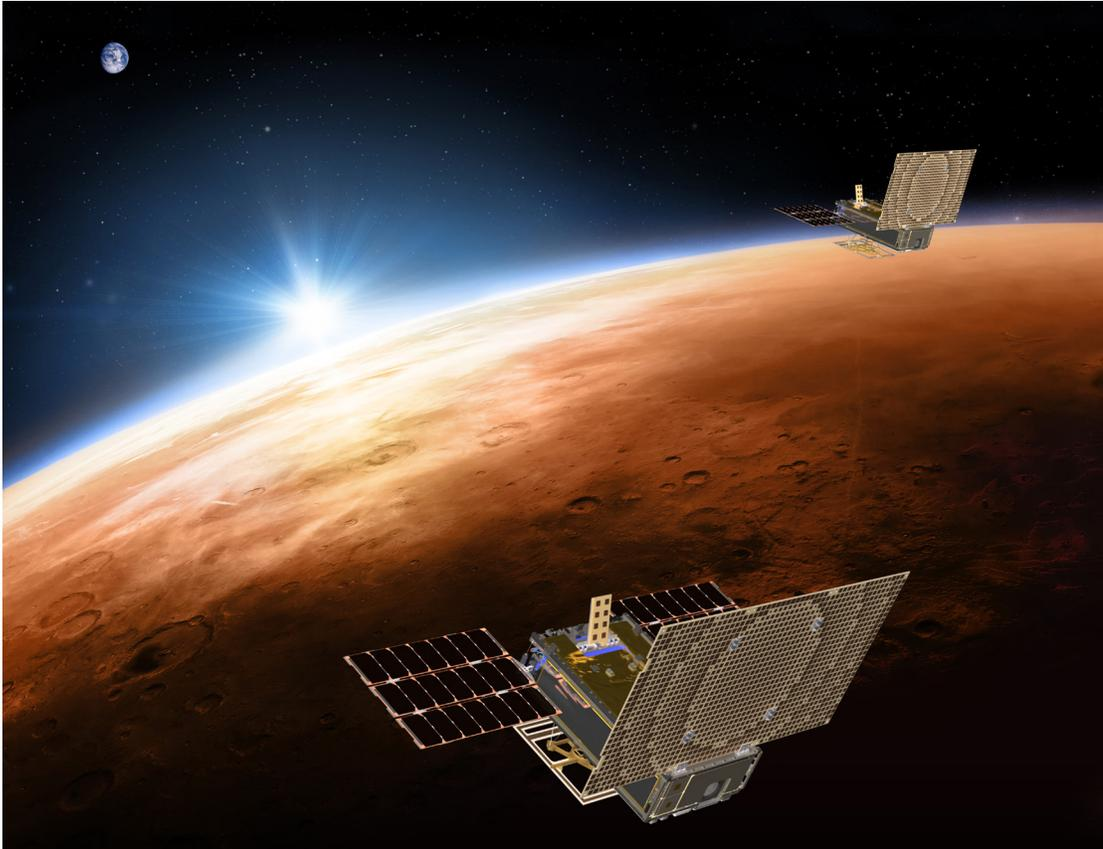
*An artist's rendering of the twin MarCO spacecraft flying over Mars with Earth in the distance. The MarCOs are the first CubeSats, a kind of modular mini-satellite, to fly to deep space. They were designed to fly along with NASA's InSight lander on its cruise to Mars. Should they make it all the way to Mars, they will provide relay of data about InSight's entry, descent and landing back to Earth. Image credit: NASA/JPL-Caltech*
