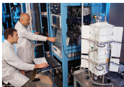
Technologists at NASA’s Glenn Research Center work with an electrically heated engineering unit of an advanced Stirling generator. Such systems could quadruple the efficiency of future radioisotope power systems for space exploration.
